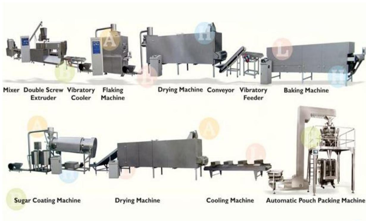
Fig 83: Corn Flakes Processing Line
