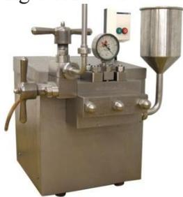
Fig 23: Homogenizer
