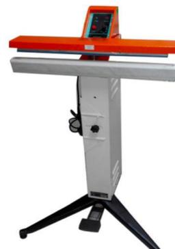
Fig 61: Foot Operated Sealing Machine
