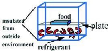
Fig 88: Indirect Contact Freezer
