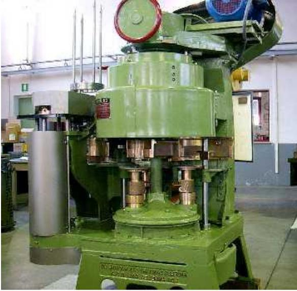
Fig 106: Can Double Seamer
