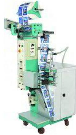
Fig 117: Fill-Seal Machine for Tomato Sauce
