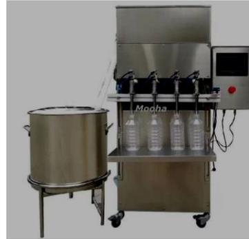
Fig 100: Filling/Bottling Unit for Juice
