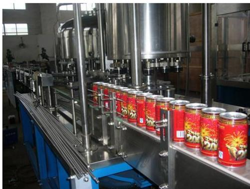
Fig 162: Can Filling Machine
